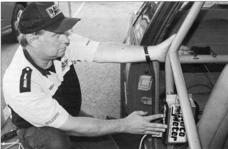
This is the Auto Meter data acquisition system on Robin Lawrence's Factory Stock car. Mounting on the roll cage as seen here puts the socket for the lap top (arrow) in the most accessible place.
