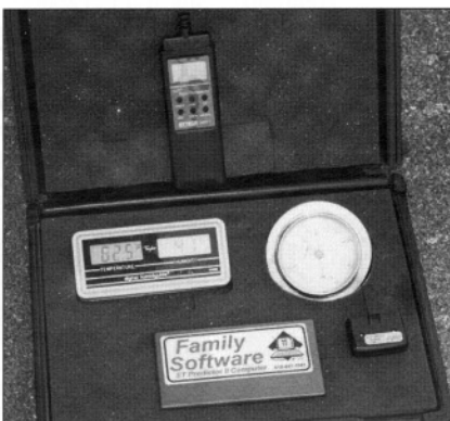
We had the necessary weather station equipment on hand to keep a track of atmospheric conditions. As it happened the amount of correction required during the test period was minimal.
