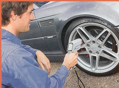
Below: Chris Witter from Performance Friction uses his gun to measure the temperature of his company's brakes. Even at 681°C they were performing well
