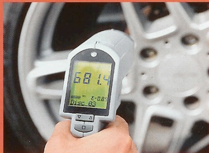
Below: Chris Witter from Performance Friction uses his gun to measure the temperature of his company's brakes. Even at 681°C they were performing well
