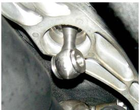
Affix shifter lower pivot to selector rod with enclosed C-clip.
