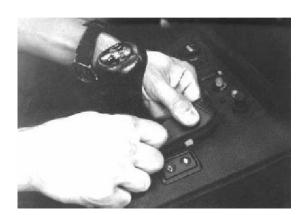
Remove the foam padding underneath the shifter boot.
