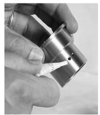
Install the unit into the carrier on top of the white bushing.
