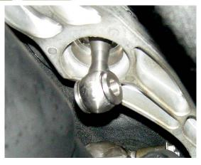
Affix shifter lower pivot to selector rod with enclosed C-clip.
