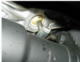
Identify and remove lower pivot clip that connects the linkage arm to the bottom of the shifter lever.
