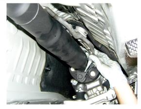
Carrier shown completely removed.
