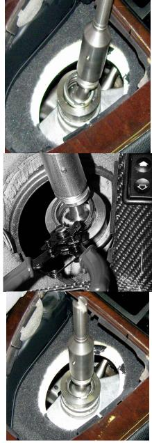
From underneath the car, insert bearing liners into both sides of shifter lower pivot bearings as shown:
