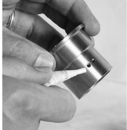
Prepare the unit by using some threadlock (included) in the threads of the holes. A small drop in each hole is all you need.
