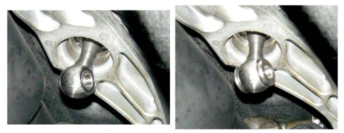
Affix shifter lower pivot to selector rod with enclosed C-clip.
