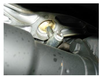
Identify and remove lower pivot clip that connects the linkage arm to the bottom of the shifter lever.
