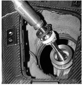
Align these four components so they fit into the pivot height adapter as shown.
