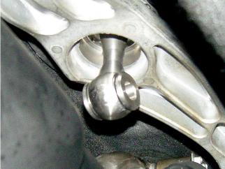
Affix shifter lower pivot to selector rod with enclosed C-clip.
