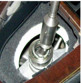
Push components in and use C-clip pliers to lock C-clip in the locating groove within the top of the pivot height adapter.
