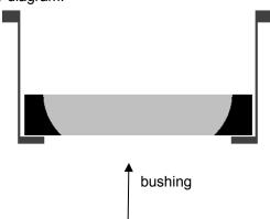
Use the included tube of grease to **lubricate the shifter** main pivot ball as shown:
