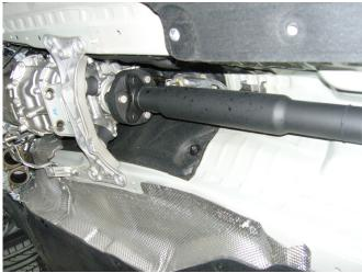
AT THIS STEP, REMOVE THE CENTER DIFFERENTIAL AND DRIVESHAFT.
