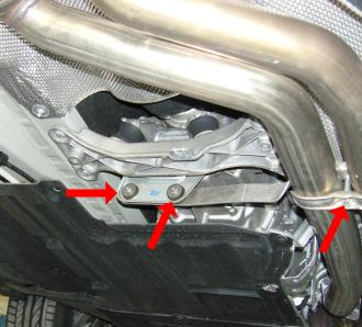
Remove exhaust support brackets as shown.
