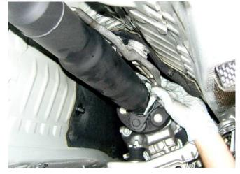
Carrier shown completely removed.
