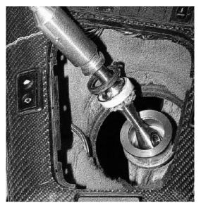
Align these four components so they fit into the pivot height adapter as shown.
