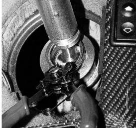
Final result. Make sure clip is securely in groove by pulling up on shifter.
