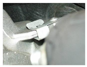
It is possible to remove these clips by pulling the bentout tab of metal with your fingers or prying out with a screwdriver.
