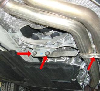
Remove exhaust support brackets as shown.
