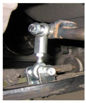
**6.** Heavily grease the swaybar pivot bushings where the anti-swaybar slides through using the grease provided. Install the greased pivot bushings onto the anti-swaybar. Remove the rear cross member bolts and use them to attach the bar with the new pivot bushings, brackets, backing plate M8 Hardware and spacer as shown below.
