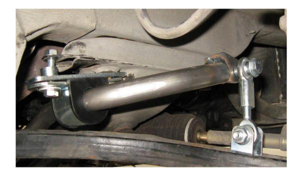
**8.** Go over the installation making sure all fasteners are tight and torqued properly. Reinstall the lower control arm rear pivot bolts, under tray and tires/wheels and slowly test drive the vehicle making sure the endlinks are the proper length and no binding or clunking occurs.
